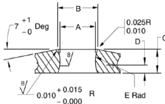
**FIGURE 4 – TITANIUM COLLAR SWAGE DIE CAVITY LIMITS (INCH)**
