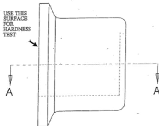
FIGURE 1 – METALLURGICAL SPECIMENS
