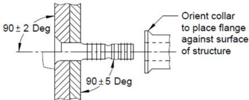
**FIGURE 3 – MAFCSLFC-MV( ) ( ) COLLAR ORIENTATION**
