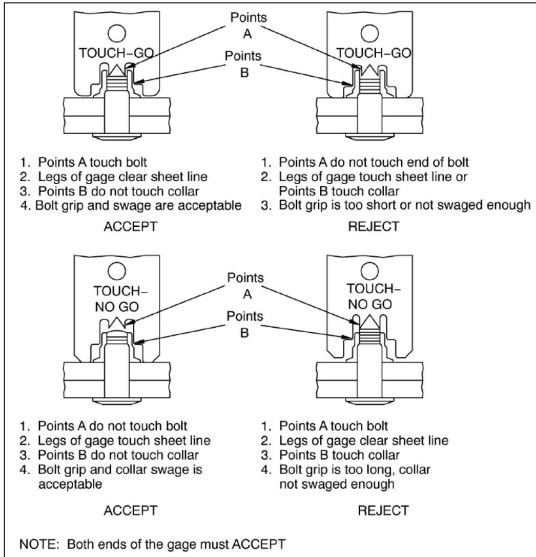
**FIGURE 6 - USE OF INSTALLATION GAGES**
